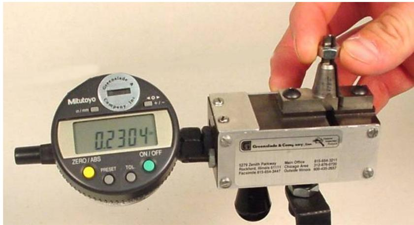
Typical Internal Variable Thread Gauge – “Bi-Point” gage
